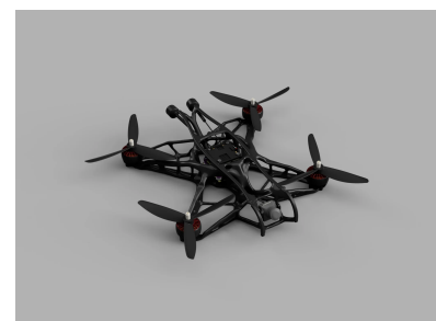
Conceptual 3D printed drone parts. We could print the whole airframe or just the camera truss.
